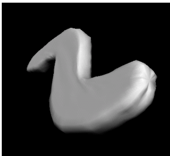
Figure B.5: The final bounding surface for the “peanut” test volume, angled to show the pinching of the mesh that resulted from uneven vertex distribution in the basis mesh.
